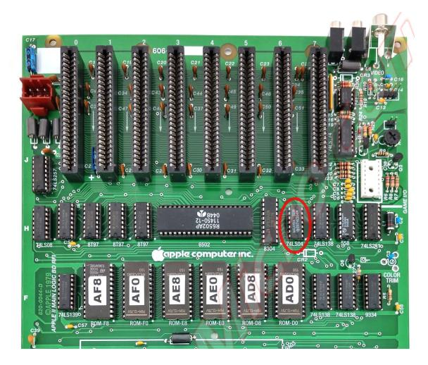
Aside from power and ground, only two pins on this chip are used: 8 and 9. To work with ROMX, you need to remove this chip and add a small jumper between these two pins. This could be done using a 14-pin DIP header or component carrier. Or you can just insert a small jumper wire into the two socket pins.
